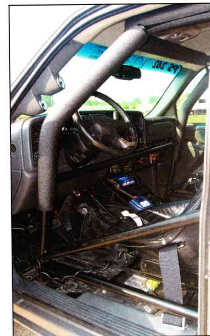
The interior of the truck is all business. A full rollcage built by DAE Motorsports out of Williamston, North Carolina, protects Buck on his 9-second quarter-mile passes. Racing seats and five-point seatbelts are also important safety features in a truck this quick.
