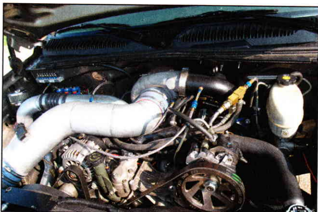
A huge (74mm) Garrett GT4202 turbo was used to provide an outlandish 65 psi to the fortified Duramax, while a dual fueler kit from ATS using Industrial Injection pumps supplies the fuel.
