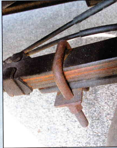
The rear has clamped leaf springs, but that's about it. Somehow this all adds up to 60-ft times in the 1.30-second range during Buck's four-wheel-drive launches.
