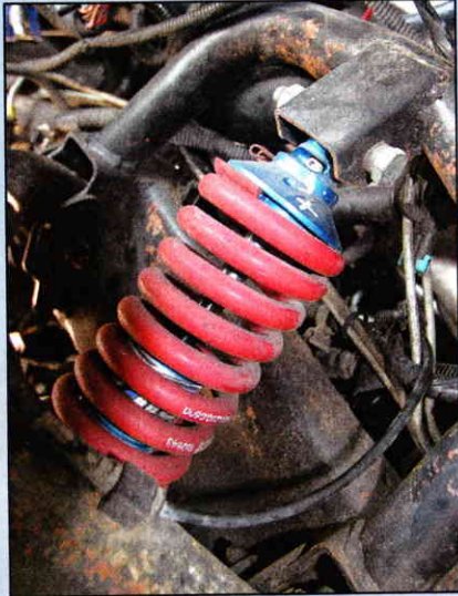
To lower the truck and aid in tuning, the front suspension was switched to coilover shocks.
