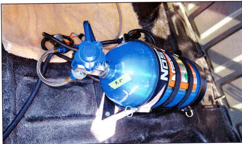
A bottle heater helps keep the truck consistent. Buck keeps the bottle at 1,100 psi and notes that bottle pressure drops to about 900 psi by the end of a run. A full bottle is emptied after only two eighth-mile passes.
