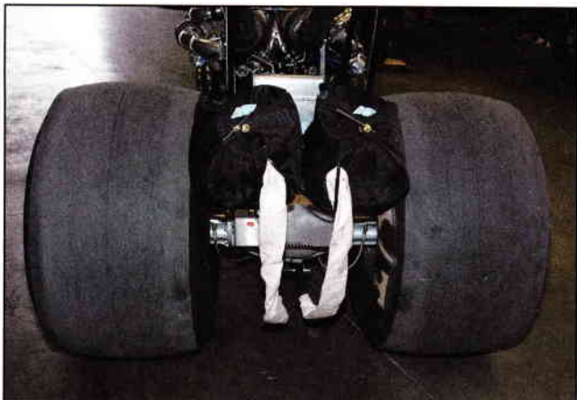
The dragster uses a Strange Engineering top-loader axle fitted with a 9 1/2-inch ring gear and spool for optimum traction and strength.
