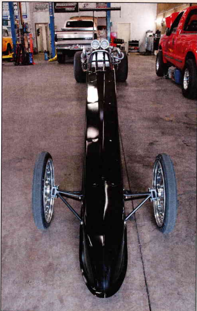
Dragsters like this are often called rails because they are so long and thin. By placing the front wheels 14 feet in front of the driver, the car can transfer weight better and becomes much more stable at high speeds.
