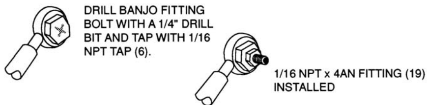
Figure 13 Schematic of “Drilled Out” Banjo Fitting
